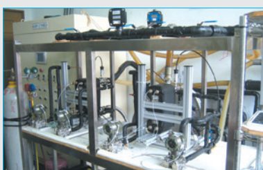
· BPHE Capacity Test Equipment
